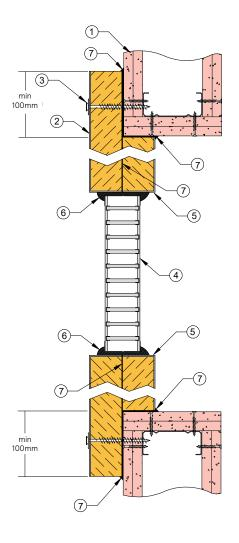
Fire rated plasterboard stud wall with TBA Firefly Intubatt containing Lorient LVH44 intumescent damper
