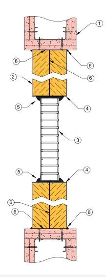
Fire rated plasterboard stud wall with TBA Firefly Intubatt containing Lorient LVH44 intumescent damper
