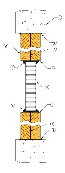
Masonry, concrete or Hebel® wall with **TBA Firefly Intubatt** containing Lorient LVH44 intumescent damper
