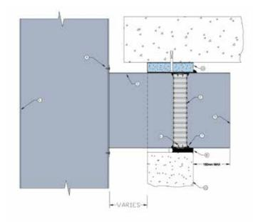
Angle free LVH44 in steel casing connected to sheet metal riser penetrating fire rated Hebel® shaft wall
