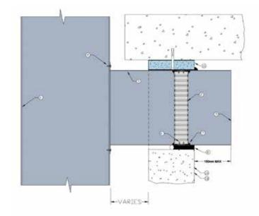
Angle free LVH44 in steel casing connected to sheet metal riser penetrating fire rated Masonry or Concrete shaft wall
