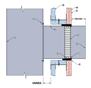
Angle free LVH44 in steel casing connected to sheet metal riser penetrating fire rated Plasterboard shaft wall
