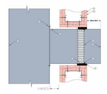
Angle free LVH44 in steel casing connected to sheet metal riser penetrating fire rated Plasterboard shaft wall
