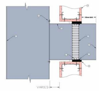
Angle free LVH44 in steel casing connected to sheet metal riser penetrating fire rated Plasterboard shaft wall
