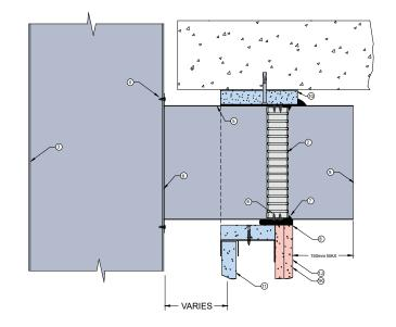
11 25mm fire rated shaft wall liner.
