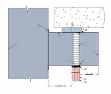
Angle free LVH44 in steel casing connected to sheet metal riser penetrating 13mm or 16mm fire rated laminated Plasterboard shaft wall
