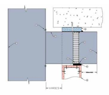
Angle free LVH44 in steel casing connected to sheet metal riser penetrating 16mm fire rated Plasterboard shaft wall
