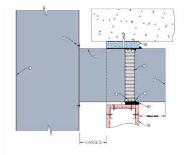
Angle free LVH44 in steel casing connected to sheet metal riser penetrating 13mm fire rated Plasterboard shaft wall
