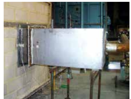
Image: AS1530.4 2014 fire damper testing
